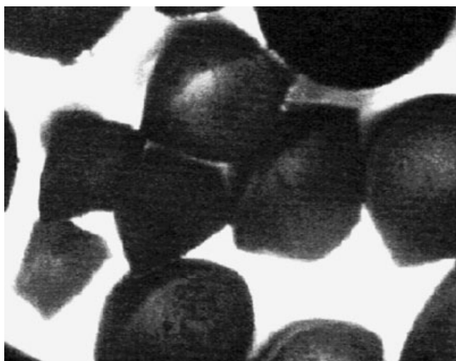
Figure 4 OM photographs of PAN as-spun fibers with jet stretch of 9.27, bath temperature of 30°C, dope temperature of 75°C, and bath concentration of 70 wt %.
